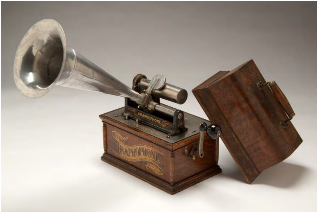
Densmore's Columbia Graphophone wax cylinder recorder. All the recordings from Standing Rock were made using this machine. Courtesy Minnesota Historical Society.
